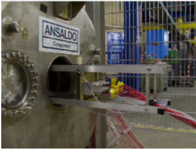
Fig. 1. Insertion of the test chamber into the magnet
