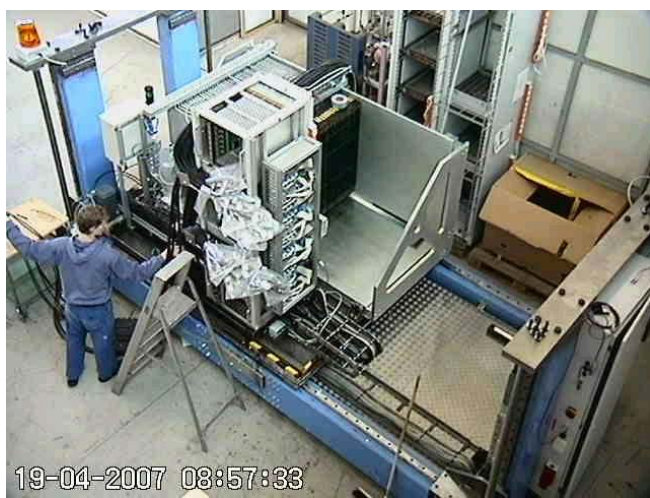
Figure 11-3: ECAL and AHCAL CALICE prototypes mounted on the motor-controlled movable stage at DESY before shipment to CERN for the summer 2007 test-beam.
