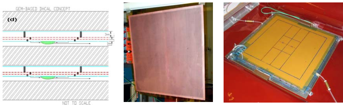
Figure 7-4 Left: GEM-DHCAL scheme. Middle: 30x30cm 2 foil. Right: Completed GEM chamber
