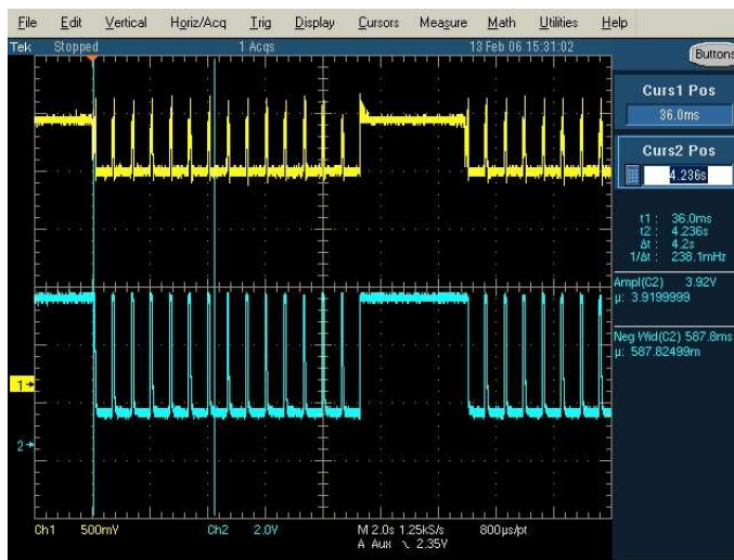
b: one readout cycle: data and power signal (note 2\text{s}/\text{div} )
