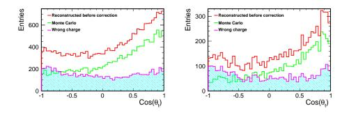
Figure 3: <u>Left</u>: Asymmetry for P, P' = -1, +1 after application of cuts in Tab. 1. The figure shows in addition the generated distribution and the events for which the *b* quark charge is incorrectly reconstructed. <u>Right</u>: The same as left but for P, P' = +1, -1
