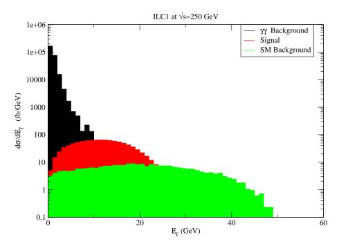
Figure 5: Distribution of missing transverse energy from  $e^+e^-$  collisions at  $\sqrt{s}=250~{\rm GeV}$  for ILC1 signal along with SM background from  $e^+e^-$  and  $\gamma\gamma$  collisions. We require 20 GeV <  $E_{vis}<50~{\rm GeV}$ . We take beamstrahlung parameters  $\Upsilon=0.02$  and  $\sigma_z=0.3$  mm.
