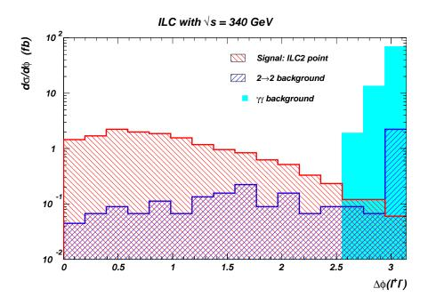
Figure 15: Distribution in transverse opening angle between isolated OS/SF leptons for ILC2 signal at  $\sqrt{s} = 340$  GeV and for SM backgrounds. We require  $E_{vis} < 30$  GeV and  $E_T^{miss} > 5$  GeV. We take beamstrahlung parameters  $\Upsilon = 0.03$  and  $\sigma_z = 0.3$  mm.
