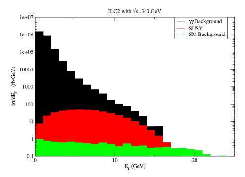
Figure 13: Distribution in missing transverse energy from  $e^+e^-$  collisions at  $\sqrt{s}=340$  GeV for signal from the ILC2 benchmark case, along with SM backgrounds from  $e^+e^-$  and  $\gamma\gamma$  collisions. We require  $E_{vis}<30$  GeV. We take beamstrahlung parameters  $\Upsilon=0.03$  and  $\sigma_z=0.3$  mm.
