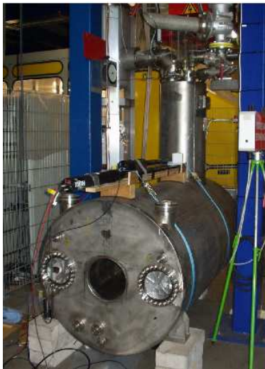
Fig. 1. The superconducting 5 T magnet in the HERA cryogenic plant and its field strength along the magnetic axis at a coil current of 1000 A.
