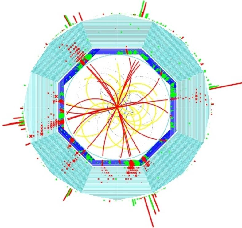
Figure 3. Simulated  $ZHH \rightarrow 6$  jets event, reconstructed following a particle flow approach. The bars at the detector circumference represent the energy of the reconstructed particles and their direction at
