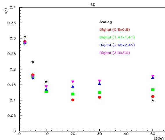
Figure 5. Simulated hadron energy resolution for a scintillator calorimeter as a function of energy for different transverse segmentations (in cm). No weighting factors have been applied in the analogue case.
