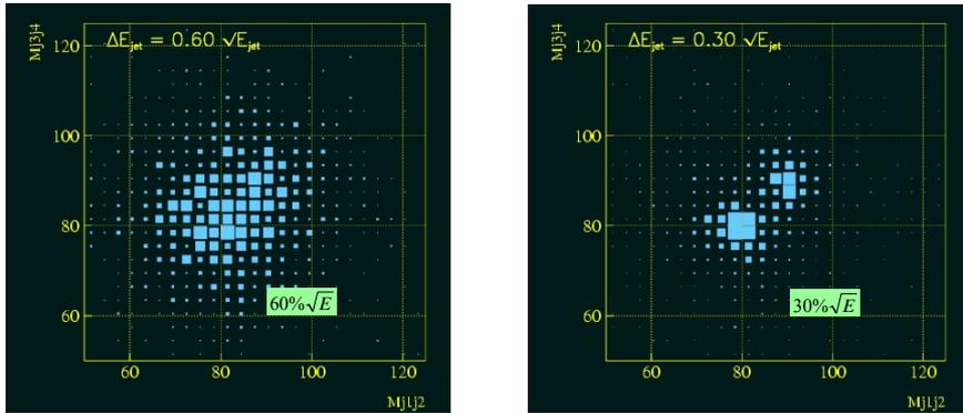
Figure 1. Reconstructed dijet masses in simulated WW $\nu\nu$  and ZZ $\nu\nu$  events, for a detector with LEP-like energy resolution (left), and with the envisaged linear collider detector performance (right).
