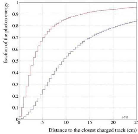
Figure 4. Fraction of photon energy carried by photons in the vicinity of charged tracks, vs. distance of closest charged track. Simulation of ZH events at 500 GeV for two different detector geometries: TESLA TDR (lower curve) and a smaller variant as proposed for Silicon based main tracking (here with  $B=6\text{T}$  and  $R=1.68\text{m}$ ). From [6].
