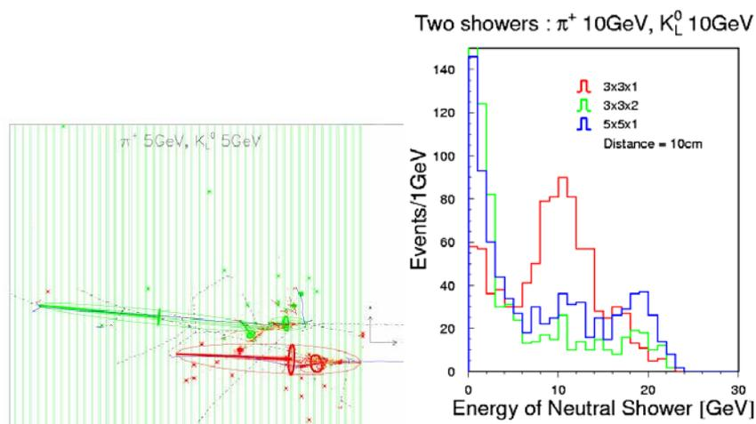
Figure 6. Reconstruction of two neighboring particles in a scintillator HCAL (left), Reconstructed energy of a simulated neutral kaon shower in the vicinity of a charged pion, for 3 different transverse granularities. The longitudinal sampling is 20 mm iron, 10 mm gap.
