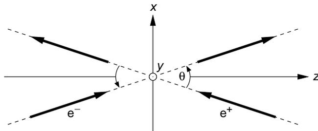
**Figure 1:** Top view of the coordinate system for a crossing angle geometry with  $\theta > 0$ . The  $y$ -axis is pointing towards the viewer. This should be the default coordinate system for all LDC detector studies.
