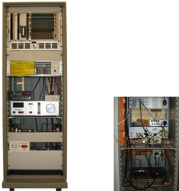
Figure 2: Slow Control Rack front and rear view. From bottom up: oxymeter, dew point instrument, flow controller, signal converter.
