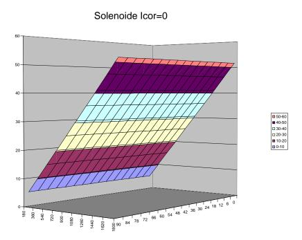
Figure 1: Configuration 1 for the coil: no correction coils, no anti-DID  $\int_{\ell_{\text{drift}}} \frac{B_r}{B_z} dz \simeq 54 \text{mm max}.$
