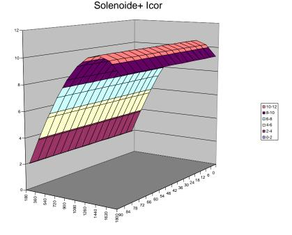
Figure 2: Configuration 2, add correction coils  $\int_{\ell_{\text{drift}}} \frac{B_r}{B_z} dz \simeq 10 \text{mm max}.$
