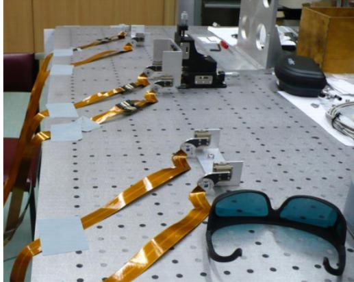
Figure 31: Left: A typical signal distribution for a semitransparent sensor. Right: A photograph of the test setup which contains six semi-transparent sensors.
