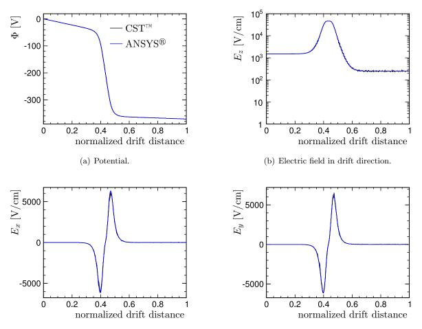
(c) Electric field transverse to the drift direction.
