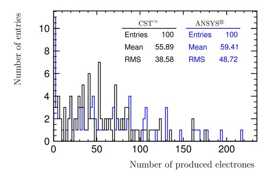
**Figure 5:** Number of produced electrons in P5 gas by a single GEM avalanche for  $CST^{\mathbb{M}}$  and  $ANSYS^{\mathbb{R}}$ .
