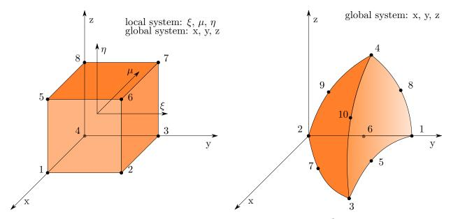
**Figure 1:** Finite elements used by CST<sup>™</sup> (left) and ANSYS<sup>®</sup> (right).
