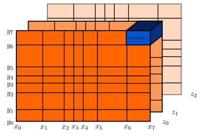
Figure 2: Sketch showing a mesh with variable element size.
