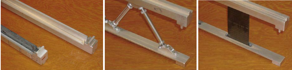
Figure 10: Small beam prototypes in 4 designs: (left) representing the cross section of the LC-TPC LP1 TPC, and a carbon fiber filled equivalent, (center) a strut space-frame design, and (right) an equivalent plate design.
