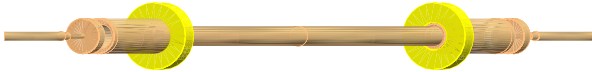
Figure 2: Schematic design of the proposed parallel shape of the beampipe. The color of the beampipe is brown, and that of LumiCal is yellow.
